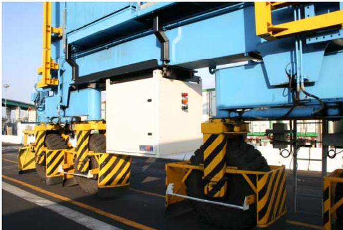
Figure 11. Flywheels installed on RTG crane
