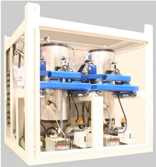
Figure 10. Two flywheel units arranged in a single package
